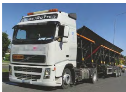
Figur 14: Stålblader transporteret under 45°
