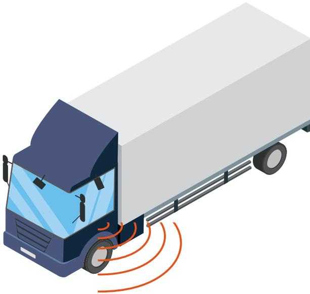
It is recommended that the volume of the audible warning, measured at one metre from the sounder, should be between 65 and 88 decibels. A combination of spoken word and white noise should be considered.
