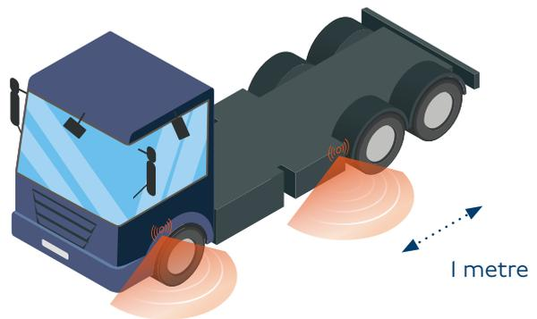
It is recommended that sensors on rigid vehicles and articulated tractor units have coverage six metres down the nearside or one metre from the rear of the vehicle (or tractor unit), whichever is smaller.
