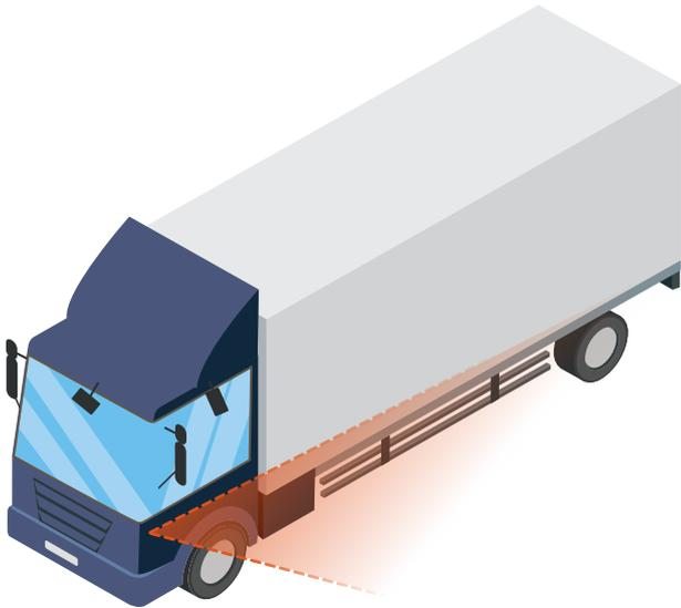
Camera monitoring systems should aim to completely eliminate or minimise the remaining vehicle blind spot at the nearside as far as is practical and possible.
